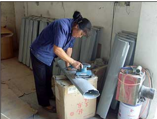
After the furnace, a worker inspects all the pieces and sands a piece if there is any defect. Then all defective pieces are reworked at the end of the batch.
