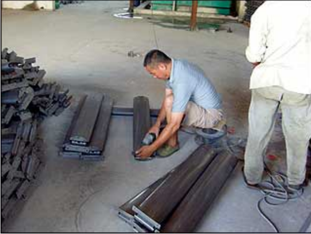
Pieces are sanded in order to improve the quality of the painting.
