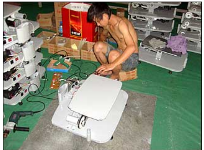
Worker performing function and noise tests at the end of the assembly line.
