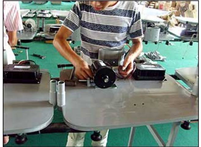
Worker fixing motor on the base
