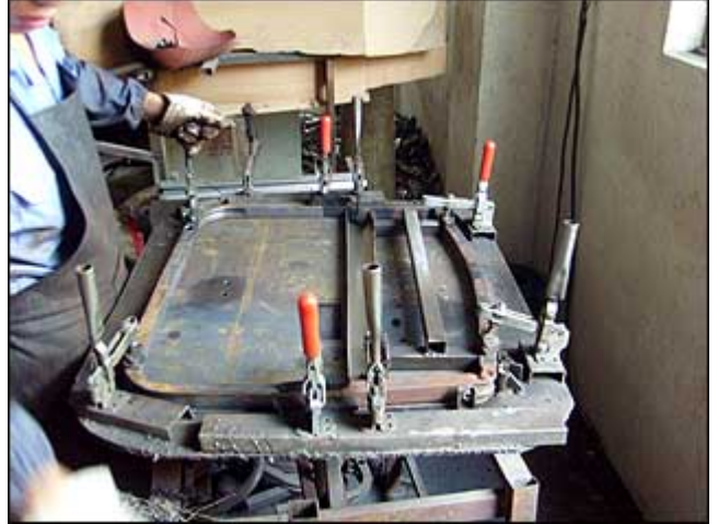
Worker is fixing all the parts of the platform before welding.
