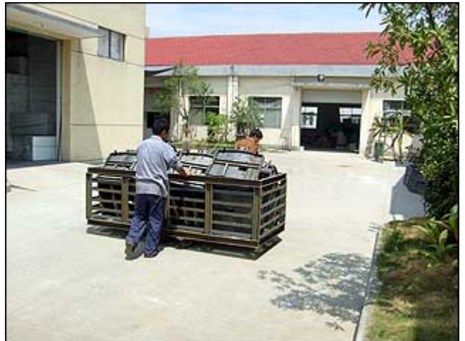
Pieces are transported from welding workshop to painting workshop by cart.
