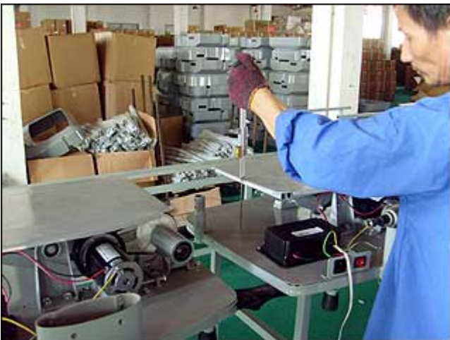
Worker testing if the base is correctly horizontal
