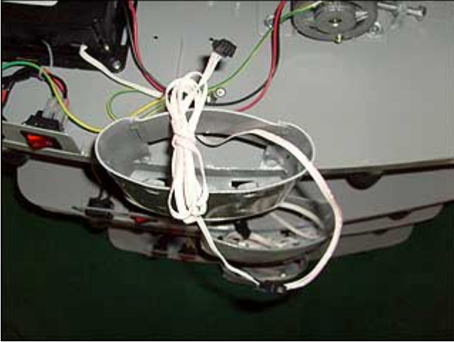
The extension wire for the connection to the panel control is plugged to the base.
