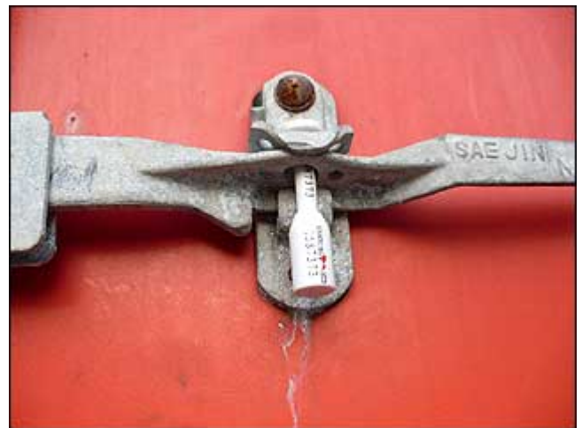
Seals details on container
